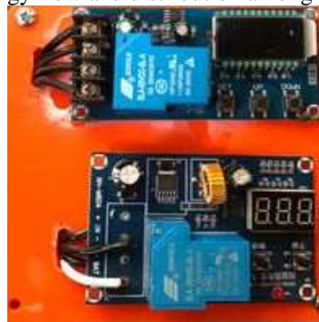
Figure 10. Pelton Wheel and Wind Turbine Charge Controller
